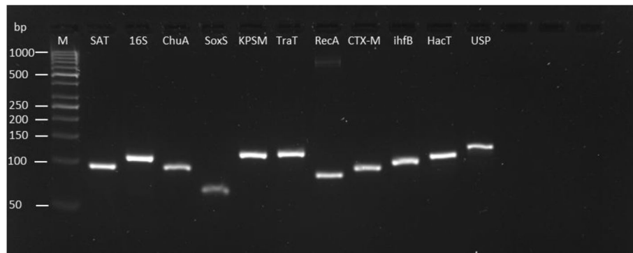
Fig. 1 The specificity of each primer pair investigated by qRT-PCR for this study. End amplified products of qPCR were visualised using agarose gel electrophoresis. All genes were detected at the expected bp size and single band was observed for each primer pair indicating primer specificity. M, Molecular Weight marker, GeneRuler 50 bp DNA Ladder (Thermofisher, UK). Products and ladder ran on 4% Agarose gel.
