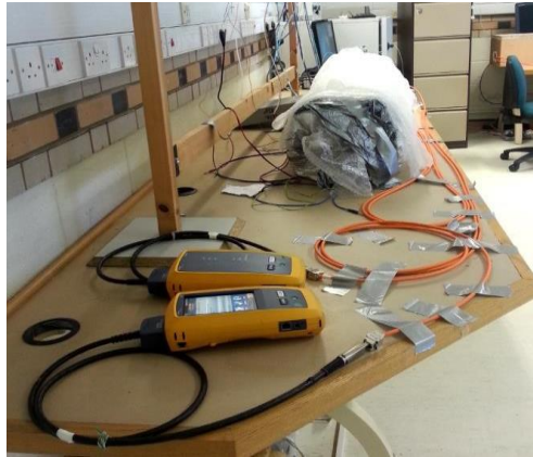
Figure 5.10: Experimental set-up for the cable portion insulation test.
