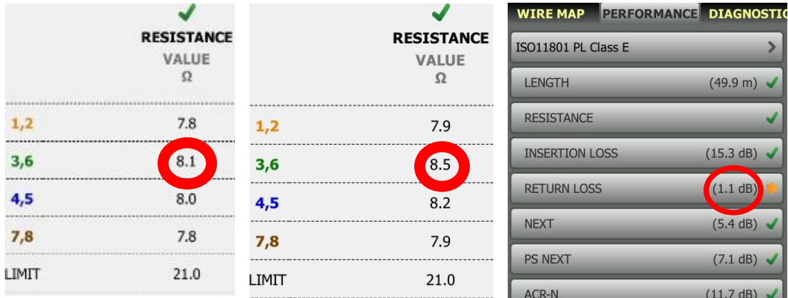
Baseline resistance (a) High contact resistance (b) Return Loss of the PL (c)
