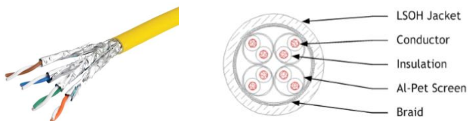
Figure 2.6: Sideways view (left) and cross section (right) of Cat 7A and 8 S/FTP cables [40]
