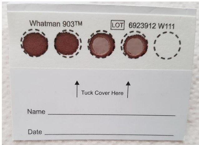
Figure 2.1. A Whatman 903 card containing four spots of dried blood and two spots punched from the marked sections.
