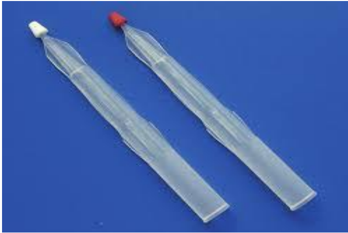
Figure 2.2. VAMS consists of a polymeric absorbent tip located on a moulded plastic handle. The unused device has a white tip, while the red tip indicates a used device as it contains dried blood (Denniff et al. , 2015).
