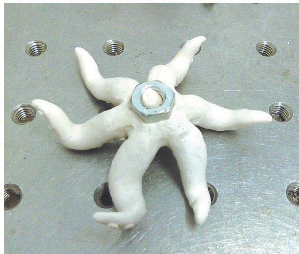
Figure 101. Plasticine figure with metal ring to secure the object from moving with a magnet.
