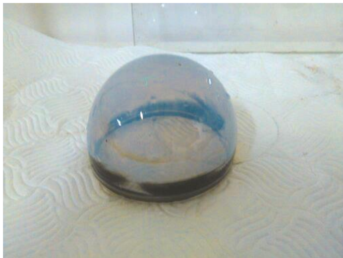
Figure 59. Fogged hemisphere after developing and bleaching.
