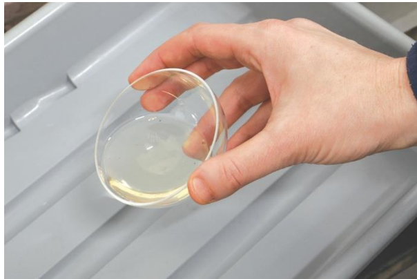
Figure 32. Coating of the gelatin by slowly moving it around in the hemisphere.
