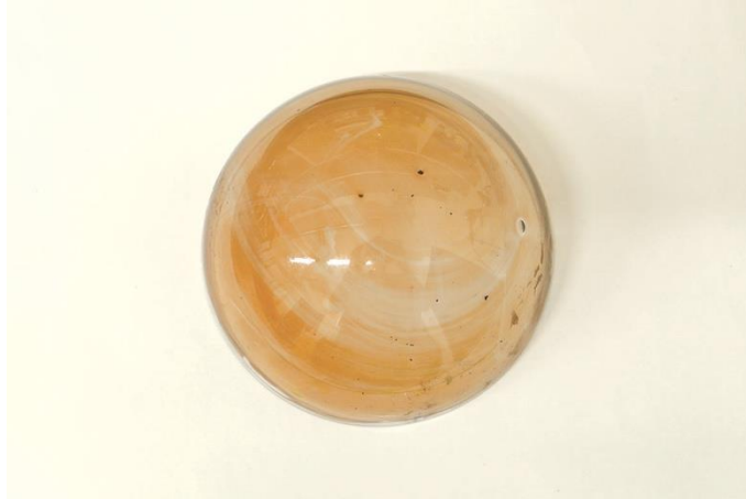
Figure 31. Hemisphere with chemical fogging.
