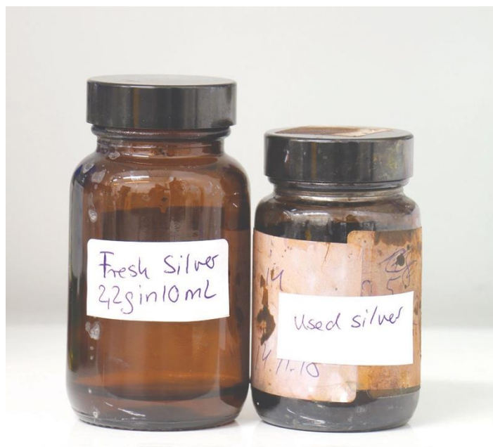
Figure 51. Two bottle system for making sure the silver nitrate solution stays clean. Silver nitrate, in forms of crystals or solution should be stored protected from light, in dark bottles, for example.
