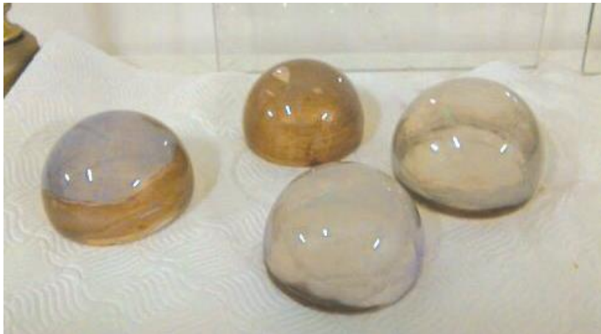
Figure 62. Fogged hemispheres from experimenting with Wash 1 and Wash 2.
