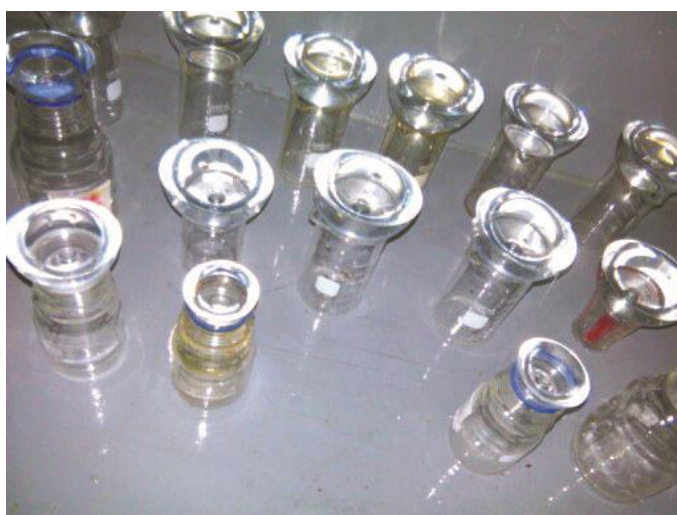
Figure 65. Hemispheres filled with sodium nitrate to be left overnight.
