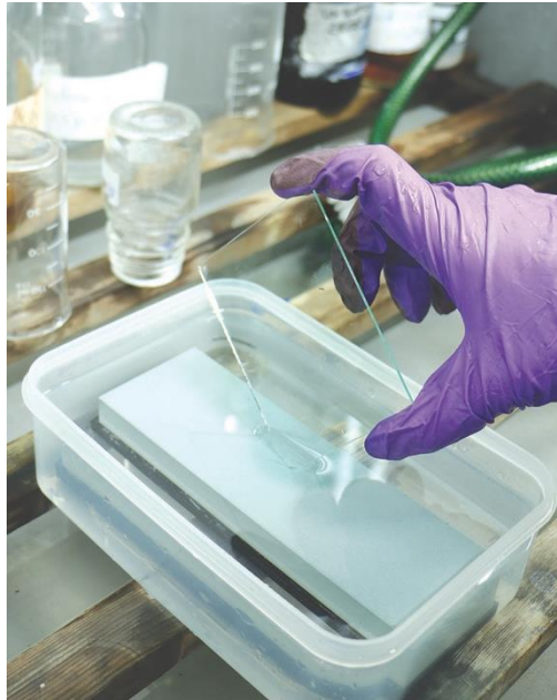
Figure 15. Glass plate and whetstone for smoothing the edges and corners.
