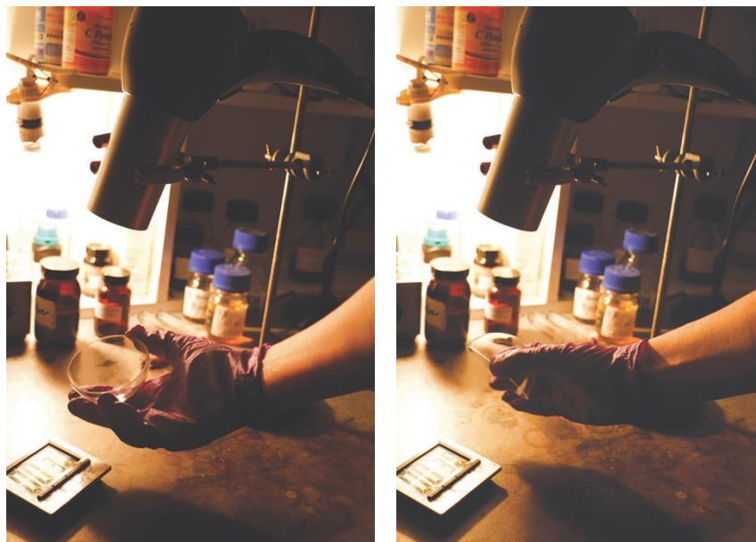
Figure 55. Drying the hemisphere after wiping under a warm air flow.
