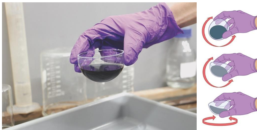
Figure 44. Applying the hardening solution to the hemisphere to harden the gelatin layer by moving it around slowly and gentle.
