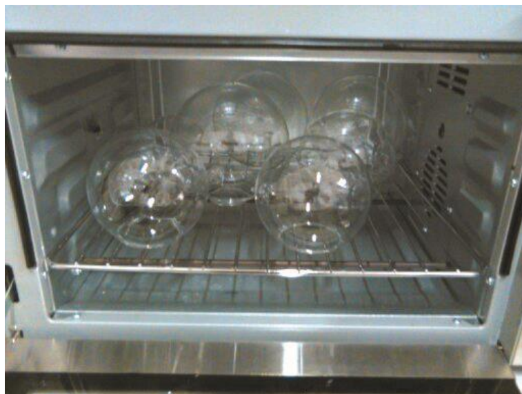
Figure 21. Bubbles in the oven for subbing.
