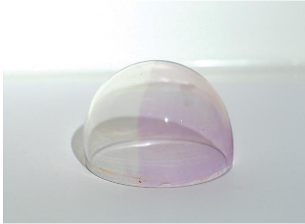
Figure 115. Bleaching of the dye stain with persulfate.
