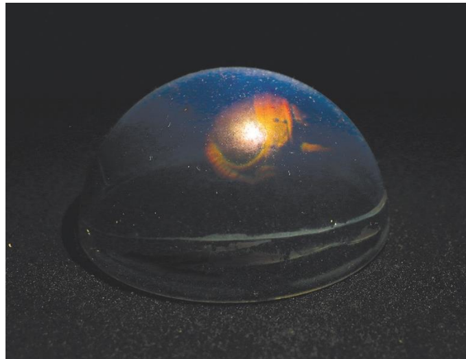
Figure 82. Lines of grain growth due to thick gelatin.
