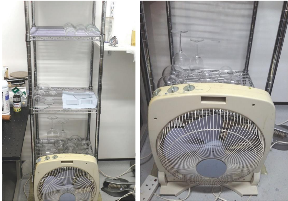
Figure 70. More effective drying on a grid.
