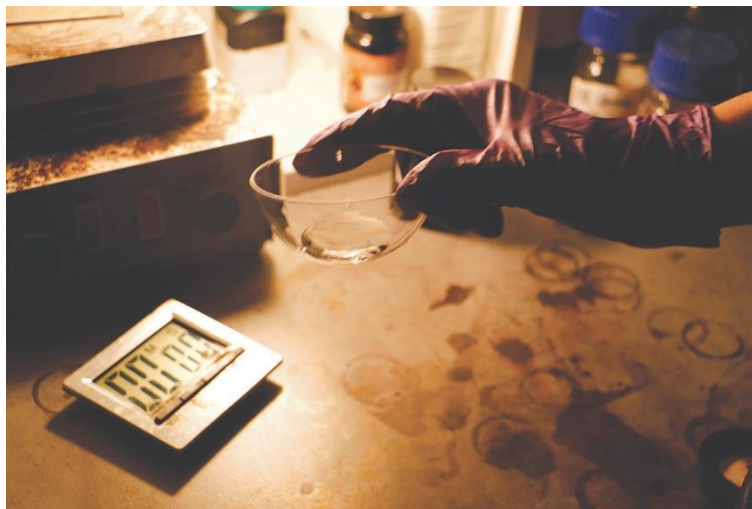
Figure 53. Moving silver nitrate around in the hemisphere slowly.
