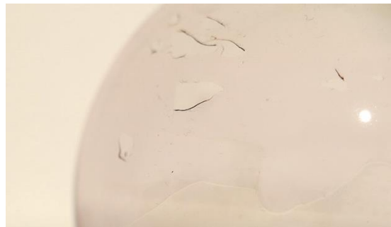
Figure 45. Scratching in the gelatin from wiping of chemicals.
