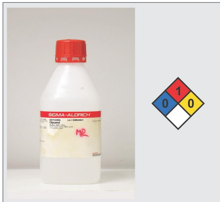
Figure 42. Glycerol, a plasticizer to reduce brittleness of the gelatin layer and promote its flexibility.
