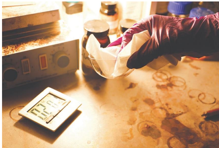
Figure 54. Wiping the hemisphere gentle to make sure spare silver nitrate is gone.
