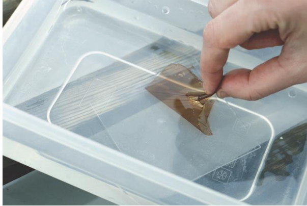
Figure 25. The gelatin can gently be lifted after the edges have parted from the substrate.
