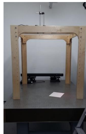
Figure 96. Overhead recording system for the recording of Hemisphere Holography.
