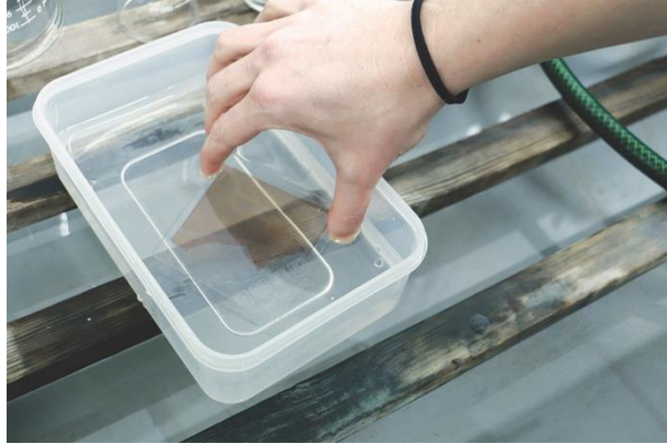
Figure 22. The plate with the unsubbed gelatin layer is submerged in lukewarm water and left until it starts to lift.
