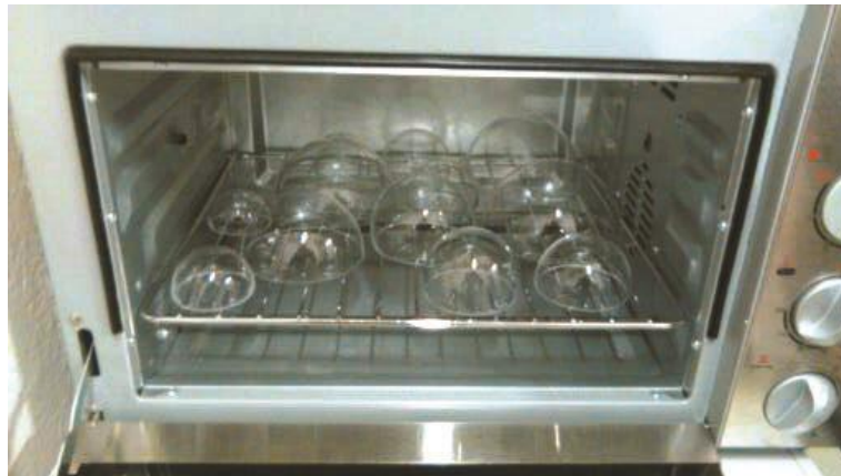
Figure 20. Hemispheres in the oven for subbing.
