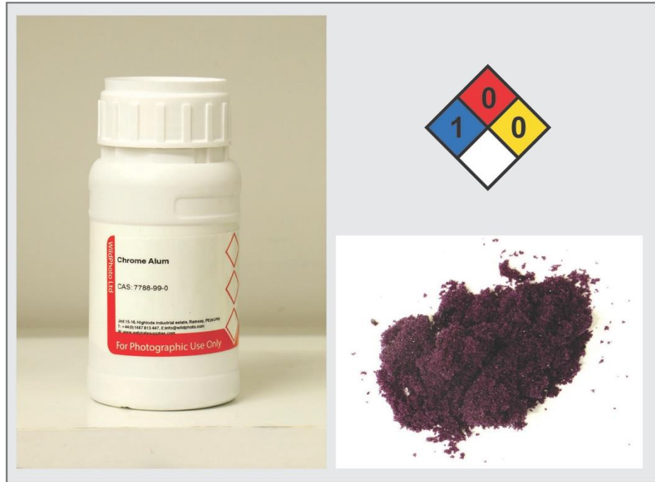
Figure 41. Chrome Alum, used to prepare the Hardener solution.
