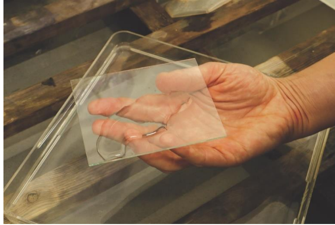
Figure 39. Gelatin is poured on a glass plate which is then slowly moved around.
