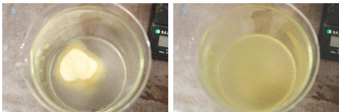
Figure 29. Gelatin just put in the de-ionized water on the left and gelatin after being in the water for 15 minutes on the right.
