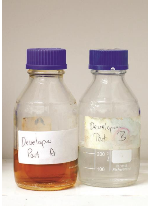
Figure 106. Part A and Part B of the developer. Part A will get darker in time.
