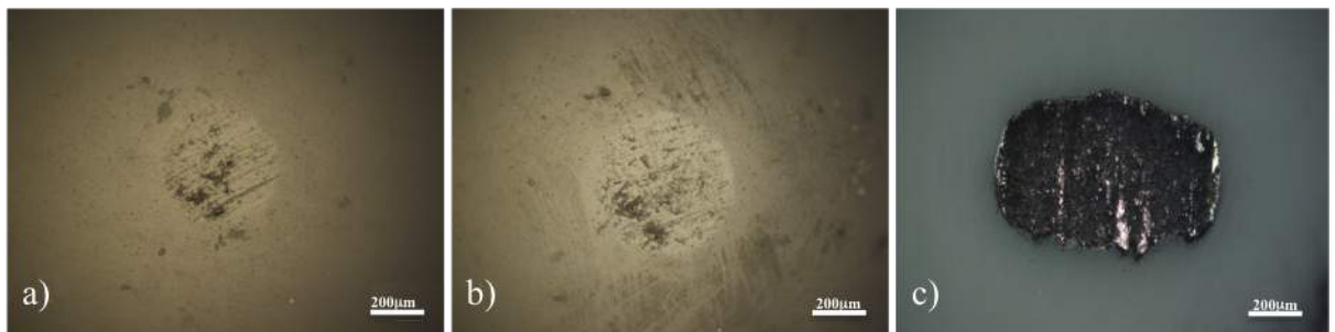
Figure 8.31: Microscopic images showing the wear scar on the alumina ball after sliding with zirconium carburised for 3h at temperature of 925^{\circ}\text{C} under 10N load after (a) 1h, (b) 2h and (c) 3h of friction and wear testing.
