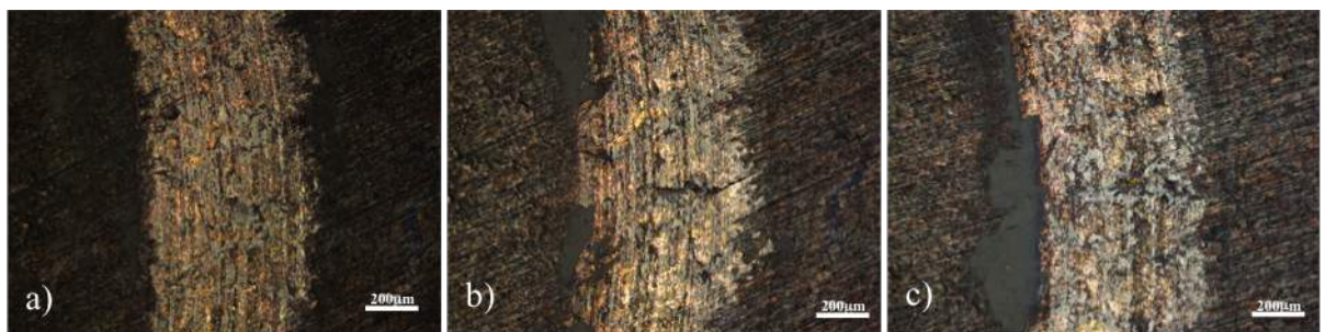
Figure 8.30: Optical microscopic images showing wear track morphology of zirconium carburised at 925^{\circ}\text{C} for duration of 40h tested under load of 10N for 3600s after (a) 4h, (b) 5h and (c) 6h of friction and wear testing.
