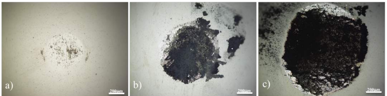
Figure 8.33: Microscopic images showing the wear scar on the alumina ball after sliding with zirconium carburised for 20h at temperature of 925^{\circ}\text{C} under 10N load after (a) 1h, (b) 2h and (c) 3h of friction and wear testing.
