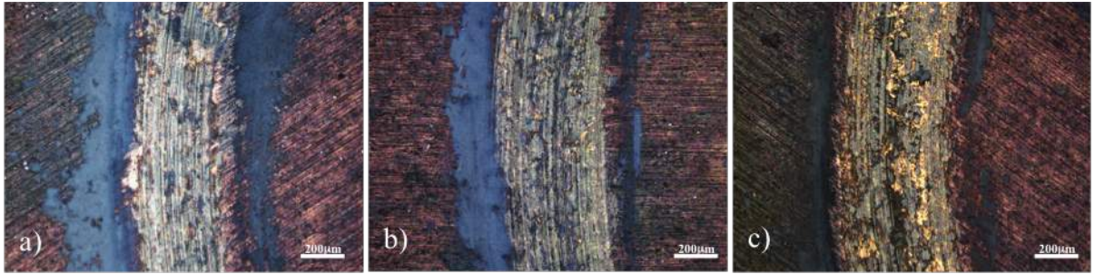
Figure 8.44: Optical microscopic images showing wear track morphology of zirconium carburised at 925^{\circ}\text{C} for 20h using composition of 20% tested under load of 10N for 3600s after (a) 4h, (b) 5h and (c) 6h of friction and wear testing.
