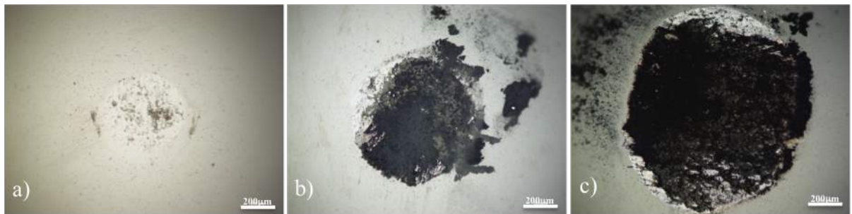
Figure 8.16: Microscopic images showing the wear scar on the alumina ball after sliding with zirconium carburised for 20h at temperature of 925^{\circ}\text{C} under 10N load after (a) 1h, (b) 2h and (c) 3h of friction and wear testing.
