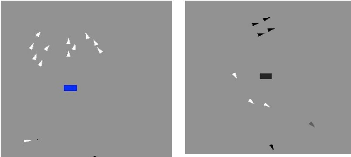
Figure A.2: Left, cohesion force binds the team members together after steering around the obstacle. Right, a screenshot shows both the alignment force and the collision avoidance rule.
