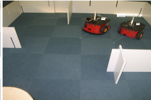
(b) Chum detects a wall, and changes the heading. Chuck aligns with Chum.
