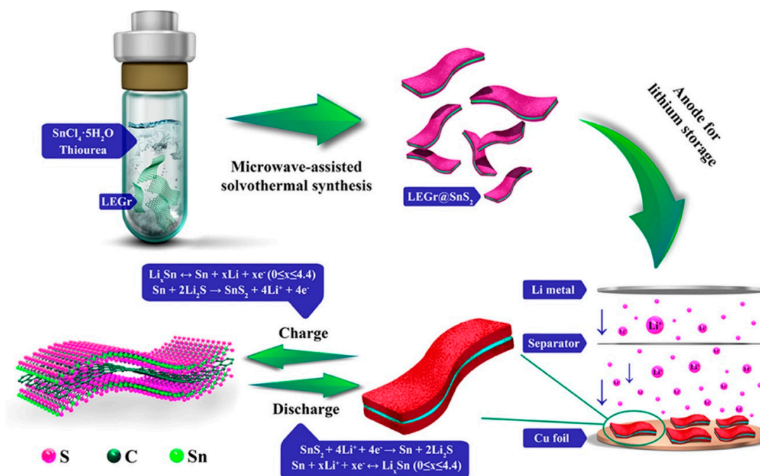
Figure 12. Schematic of the synthesis method and applications of LEGr@SnS 2 heterojunctions. Reproduced with permission from [121].
