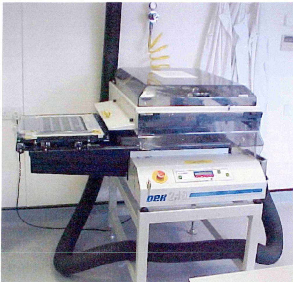
Plate 2.1: A DEK 248 semi-automatic precision screen-printer.
