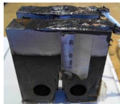
Fig. 6. (a) Schematic of a C(T) specimen with bonded strain gauge (b) strain gauge insulation during CF tests.
