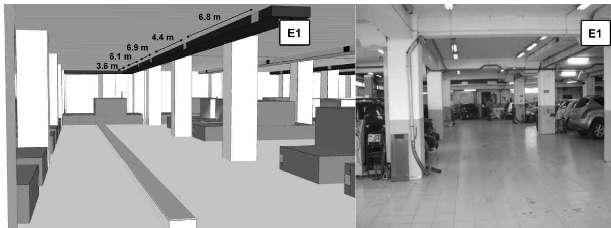
Figure 2. Layout of the western orientation rectangular vents in the E1 branch and location of the “artificial” CO linear mass source (left) and respective photograph (right).
