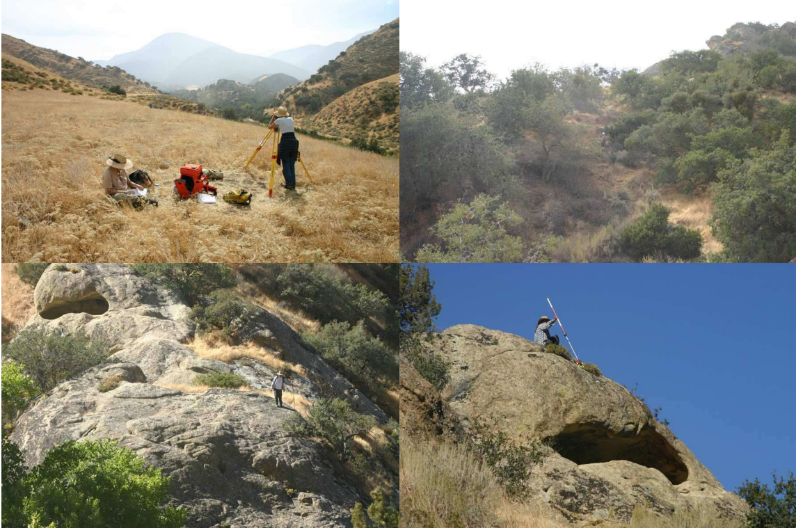
Figure 1. Mapping Pleito using a Topcon total station.
