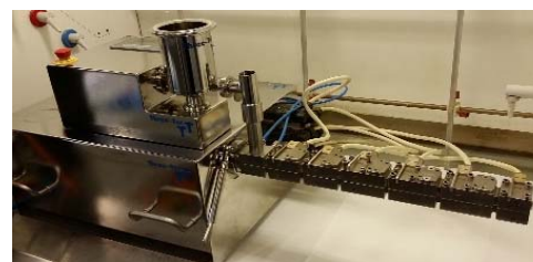
Figure 1: Laboratory scale 12 mm, 40:1 L/D Twin Screw Extruder that fits into a standard fume cupboard.
