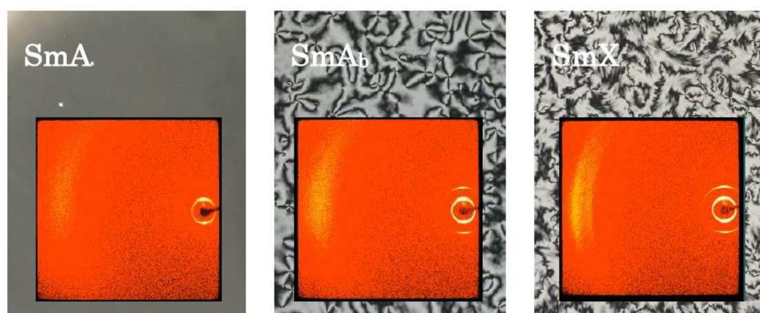
Figure 5. POM images and corresponding X-ray diffraction patterns obtained for CB6OBA:10OS in the SmA , SmA_b and SmX phases (left to right).
