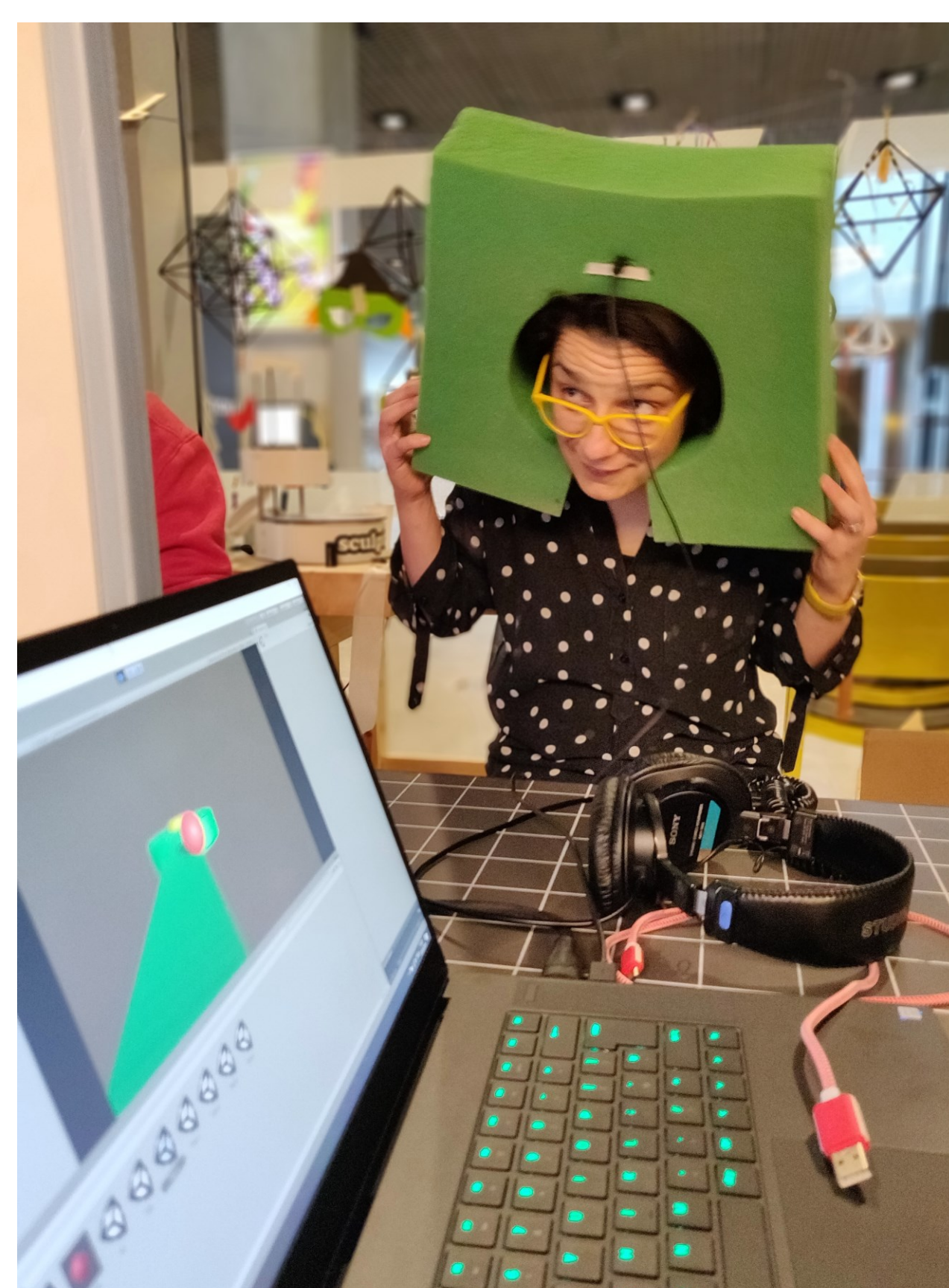
Figure 4: Controller workshop at Counter Play '19. The controller uses orientation sensors and was placed on players heads using tilt as the input. Augmenting the level based on how much the player leaned their head.
