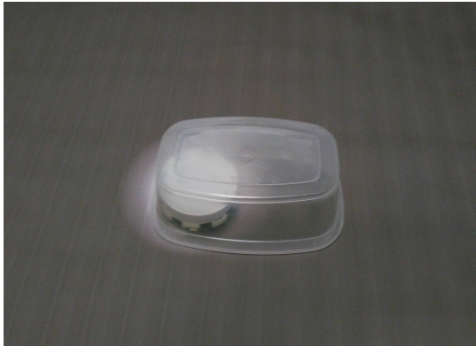
Fig. 4. The Elisa-3 robot covered with a plastic container, to induce stress in conditions 2–6. The robot was trapped with a food resource (light floor patch) so that it did not die through lack of energy while trapped.
