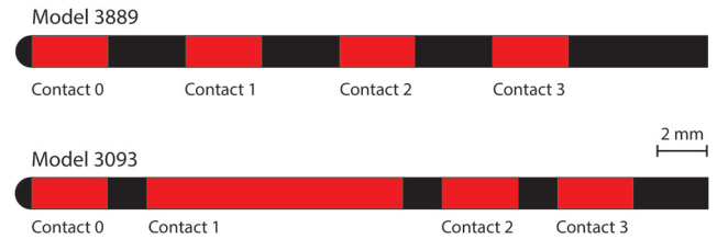
Fig. 3 Schematic representation of the two models of quadripolar electrode represented in this study. Model 3889 (top), diameter of 1.27 and 3 mm long contacts separated by 3 mm. Model 3093 (bottom), diameter of 1.27 mm, three 3 mm long contacts and one 10.2 mm long contact, all separated by 1.5 mm
