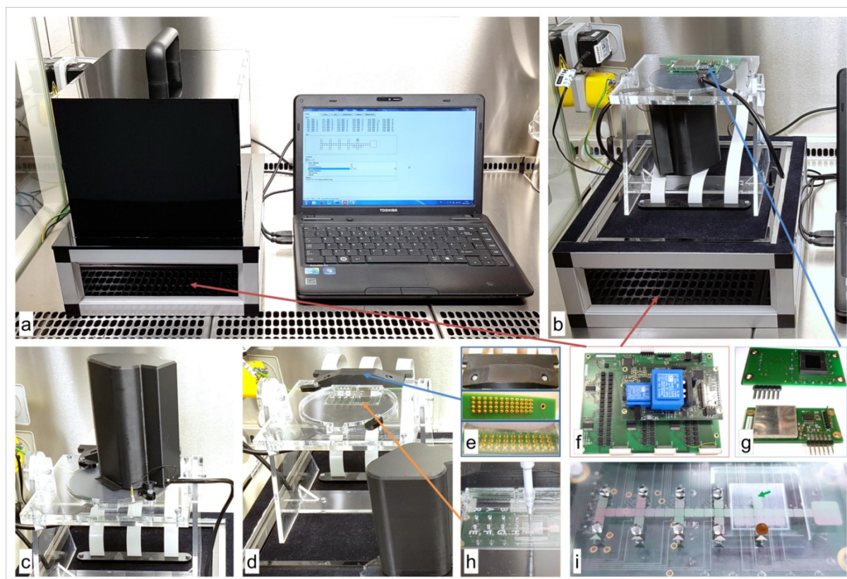
Figure 3. The digital microfluidics platform. (a) Overview of the all-integrated platform in operation; the dark Faraday cage, in which the EWOD operation, the magnetic separation and the detection are performed, allows a minimal electromagnetic interference; the platform is connected to a computer running the bespoke software interface controlling droplet operation. The approximated dimensions of the unit are 26 x 30 x 30 cm 3 . (b) The platform with the chamber opened and its rotating stage in running position (magnet at the bottom). (c) The platform with rotating stage in droplet loading position (magnet on top). (d) The platform in droplet loading position with the lid (magnet attached) removed and the loading deck on. (e) Sprung-loaded connector (pogo pins) for electrical connection with the EWOD plate. (f) Integrated electronics: the top board comprises the wave generator and the bottom board encompasses the control electronics. (g) The photodetector board comprising pre-filters and shielding case. (h) Manual pipetting of droplet through the droplet loading deck. (i) EWOD chip comprising the loaded droplets, the green arrow points to the detection site.
