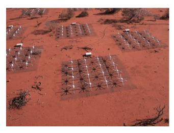
Figure 1. Examples of the MWA's aperture array antenna 'tiles', each comprised of a  $4 \times 4$  grid of individual bow-tie dipoles (Image credit: MWA Project, Curtin University).
