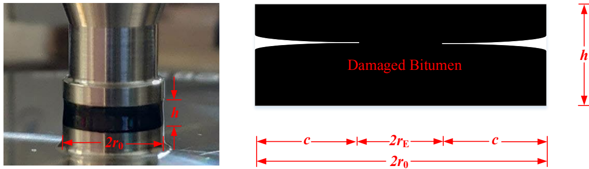
Fig. 1. Trimmed configuration of an undamaged cylindrical bitumen sample and schematic side view of the damaged cylindrical bitumen sample in DSR tests
