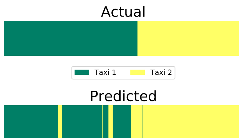
Figure 7. Prediction of the value of \tau_t corresponding to the taxi identity on the test. The top plot shows the sample labels, whereas the bottom plot shows the predicted \tau_t values using the AI-HMM with an accuracy of 93%.
