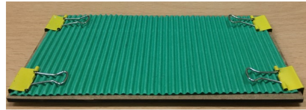
Fig. 7. Rippled paper with almost perfect sinusoidal texture patterns.
