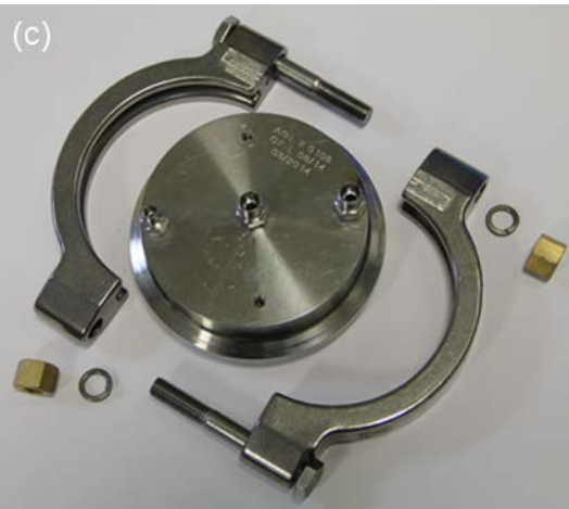
Figure 159. The (a) loaded membrane cell is (c) clamped with a (b) 4.0" high pressure clamp to give the (d) fully assembled membrane cell.
