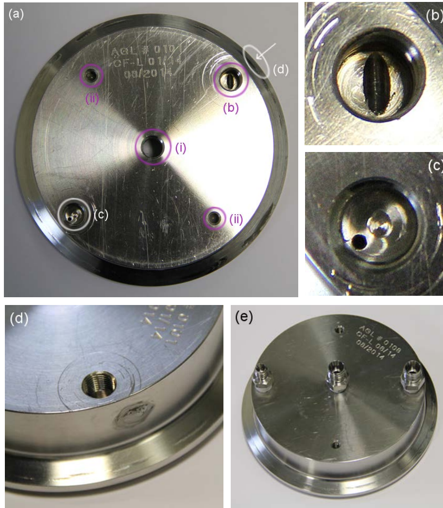
Figure 155. Membrane housing cell upper half outside (see Figure 156 for the inside). (a) Overview with (b) angled feed inlet, (c) permeate outlet and (i) retentate outlet as well as (ii) optional threads for attachment to a frame. (d) The angled feed inlet is drilled from the outside and the gap between feed tube and outside subsequent welded closed. (e) Fittings are inserted into the topside via 1/8" NPT threads.
