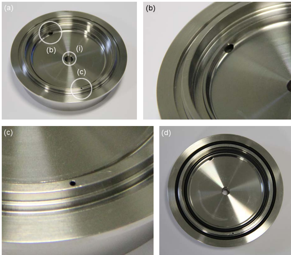
Figure 156. Upside-down view of the membrane housing cell upper half inside (see Figure 155 for the outside). (a) Overview with (b) angled feed inlet, (c) permeate outlet and (i) retentate outlet. (d) Overview with inner and outer O-rings inside their respective grooves. The inner O-ring seals the feed/retentate compartment against the permeate compartment, i.e. it separates the compartments on either side of the membrane. The outer O-ring seals the permeate compartment from the atmosphere outside the cell.
