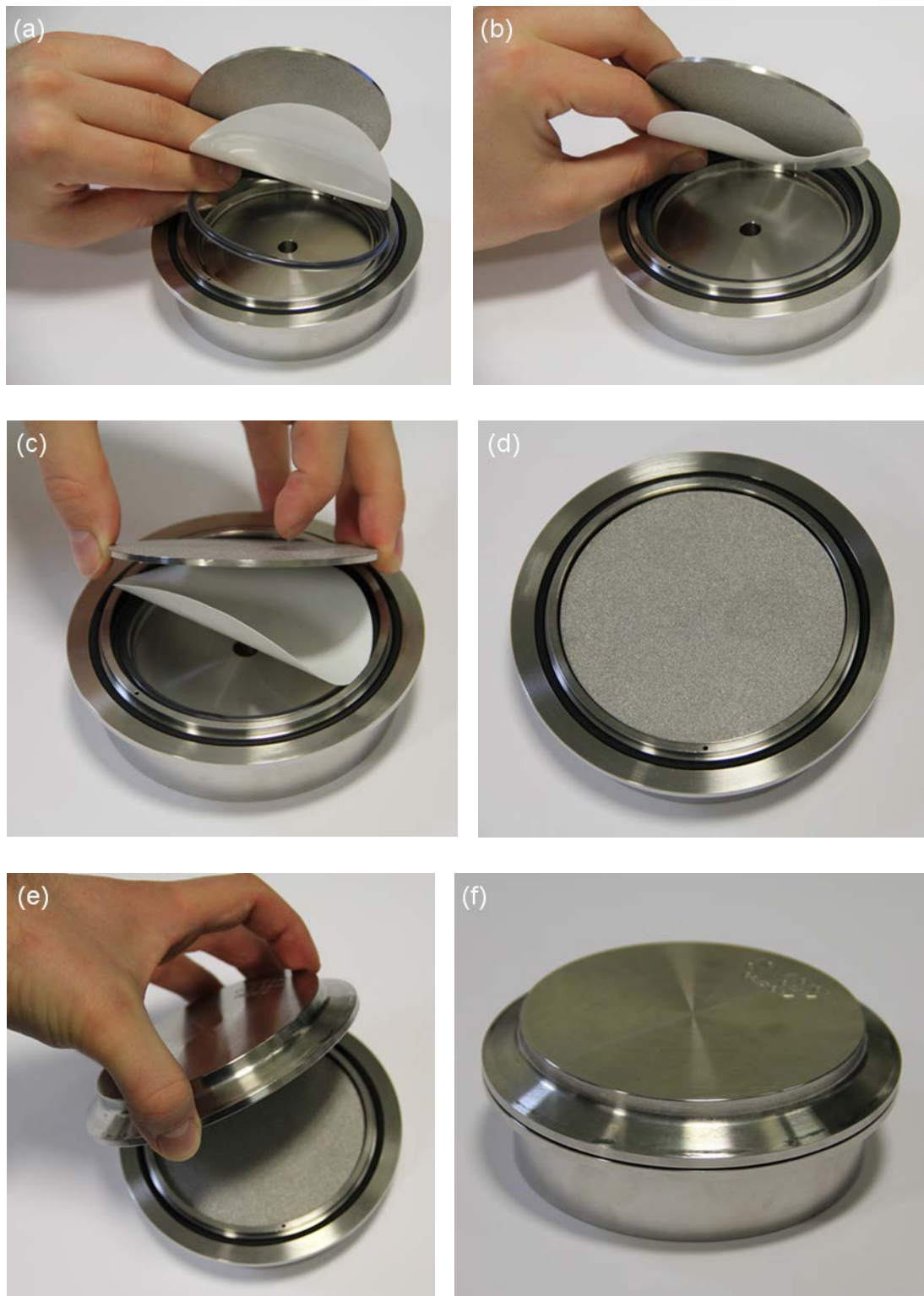
Figure 158. Step 1 - 6 (a – f) of membrane cell assembly in upside-down position. The flat white sheet of polymeric material visible in Step 1 - 3 is a PEEK membrane coupon; the PEEK active layer is facing towards the feed and retentate side (towards the O-ring) and the polypropylene backing is facing towards the permeate side (towards the sintered steel disc).
