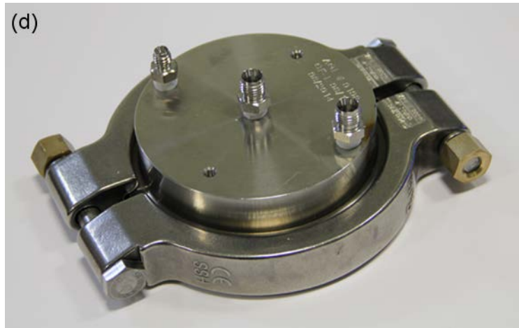
Figure 159. The (a) loaded membrane cell is (c) clamped with a (b) 4.0" high pressure clamp to give the (d) fully assembled membrane cell.
