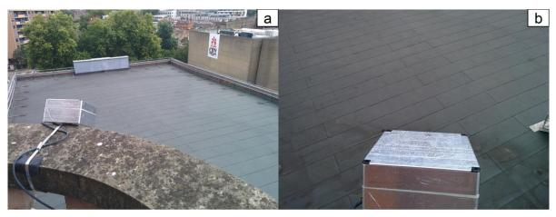
Figure G-1. Enclosed longwave infrared camera (camera C7) installed at the CUB site for atmospheric correction evaluation with its "short" roof-camera path length (a) mounted on a bell tower to the southwest of the target roof. Images taken on 7<sup>th</sup> September 2017.
