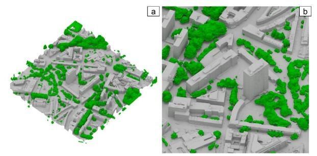
Figure D-1. Urban surface geometry as (grey) a vector-based 3D surface model and (green) a voxel-based model of vegetation canopy elements for the central London (UK) study area (Chapter 3 and Chapter 4) rendered using Blender (Blender, 2018).
