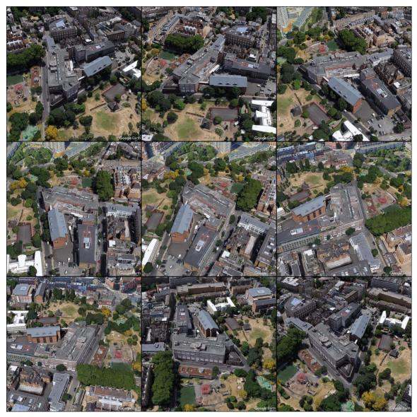
Figure D-2. Sample images captured by Google Earth using a pre-programmed Google Earth "tour". Images are used to create a dense point cloud "tile" in Agisoft PhotoScan Professional (Figure D-3).
