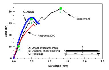
Fig. 3 Comparison of observed and predicted load-deflection responses.
