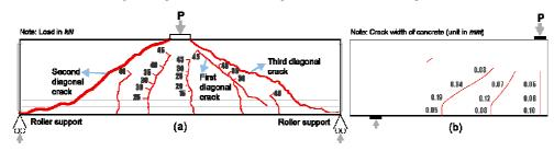
Fig. 4 (a) Crack pattern observed after failure and (b) predicted crack pattern from Response 2000.
