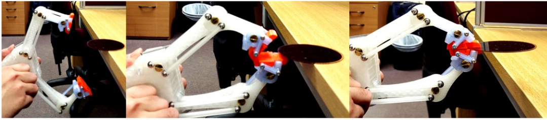
(c) Wafer, 9.5g, dimensions: \Phi 76\text{mm} * 0.8\text{mm}
