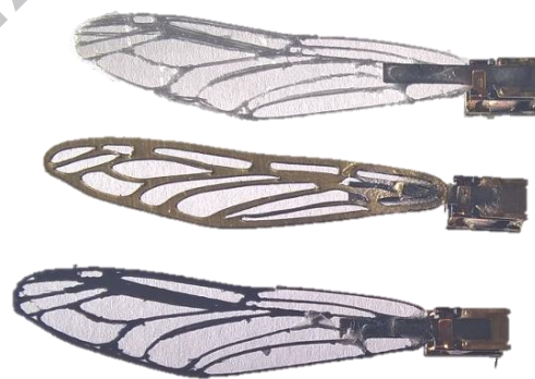
Fig. 2 Wing frame materials of PLA, acrylic and ABS respectively.
