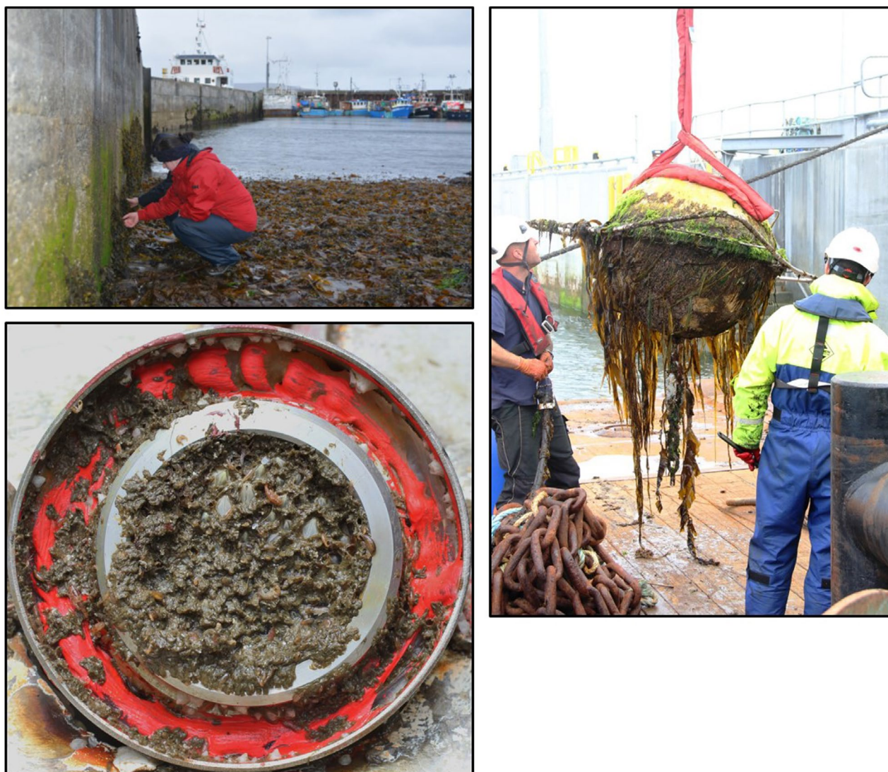
Figure 2. Field survey images (clockwise from upper left): sample identification at Tingwall harbour; Waverider buoy from Billia Croo; and camera lens on acoustic Doppler current profiler (ADCP), Fall of Warness.
