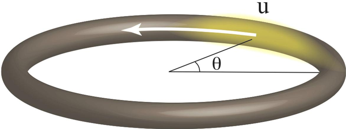
FIG. 1. The tightly confined ring with radius  $R$  circumferentially traps the Bose-Einstein condensate such that the dynamics is effectively one-dimensional along the azimuthal or  $\theta$  direction. The chiral soliton of velocity  $u$ , indicated by the yellow region, is only allowed to travel in one specific direction given by the parameters of the current nonlinearity.
