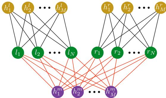
FIG. 1. Sketch of the employed neural network. The visible layer is in green and hidden layers are in light brown and purple. There is a hidden layer for the row indices  $l_i$  and the column indices  $r_i$  of  $\rho$  ( $i = 1, 2, \dots, N$ ) with hidden neurons  $h^l_j$  and  $h^r_j$  ( $j = 1, \dots, M$ ). A further hidden layer with neurons  $h^m_k$  ( $k = 1, \dots, \tilde{M}$ ) is responsible for the mixing, cf., [31].
