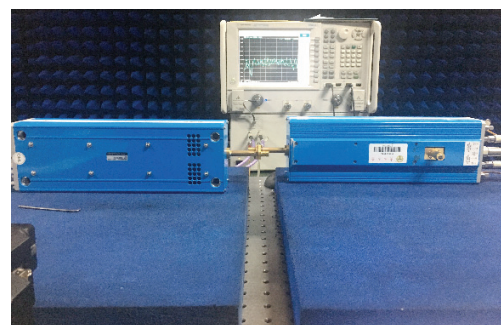
FIGURE 8. Measurement setup for the W-band extraction.
