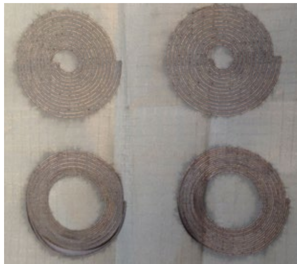
Fig. 4 Patterned conductive coils were cut by a laser cutter.
