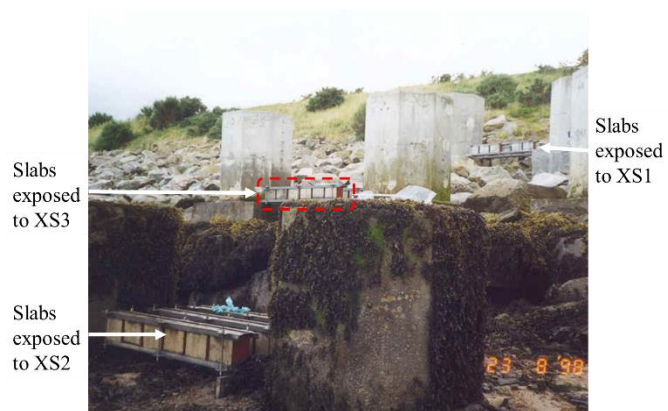
Fig. 3. Frames containing slabs installed at Dornoch field site in XS1, XS2 and XS3 positions.
