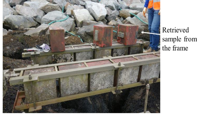
238 Fig. 5. Concrete slabs retrieved from frame in XS3 environment.
