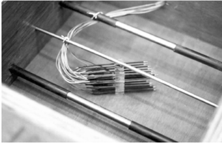
Figure 4. Covercrete electrode array (McCarter et al. 1992)
