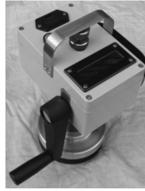
Figure 12. The Limpet Pull off Test
