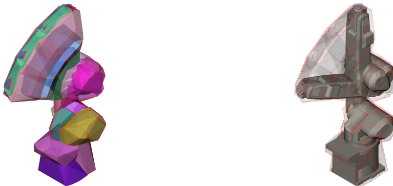
(a) A bounding set of convex polyhedra tightly encloses a swept volume of a robot motion. (b) Overlay on start and end poses of the path.
