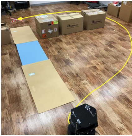
Fig. 6. The setup for the second scenario. The goal is shown as a red cross in the image. Two paths are available to the goal; the shorter one contains soft ground, the longer one is entirely hard floor. When carrying a payload, the robot avoids travelling over the foam.
