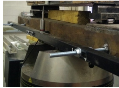
307 Figure 7. Four-point bending test setup a) Instron machine, b) Loading rig, supports and LVDT positions, c) 308 loading rig d) support e) LVDT holder
