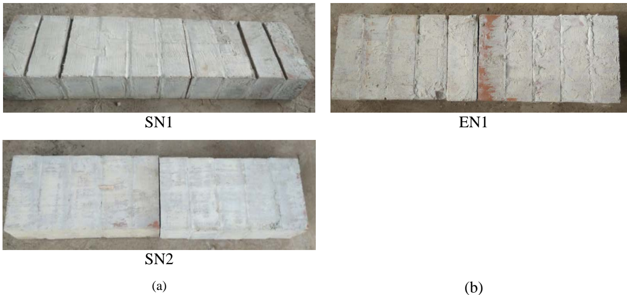
396 Figure 14. Crack patterns at failure exhibited by the un-strengthened specimens when subjected to loading rates 397 of a) 1 mm/min and (b) 200 mm/min.
