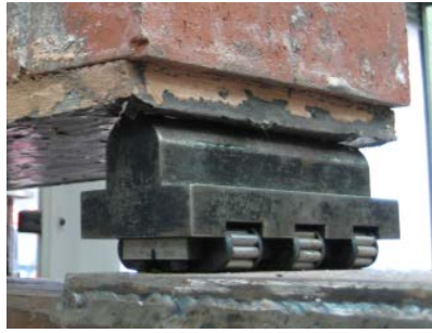
307 Figure 7. Four-point bending test setup a) Instron machine, b) Loading rig, supports and LVDT positions, c) 308 loading rig d) support e) LVDT holder
