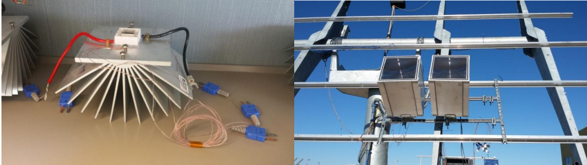
139 140 Figure 1: A CPV receiver assembly using an EMCORE solar cell bonded on a DBC and an aluminium heat sink (left) 141 and a photograph of two DDM-1090 \times monomodules mounted on the solar tracker in Albuquerque, NM (right). 142
