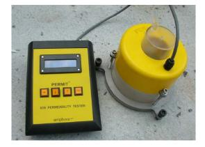
Figure 4: The PERMIT ion migration test apparatus
