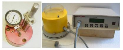
(a) CLAM water tester(b) Autoclam permeability test systemFigure 3: Different versions of CLAM permeability tests
