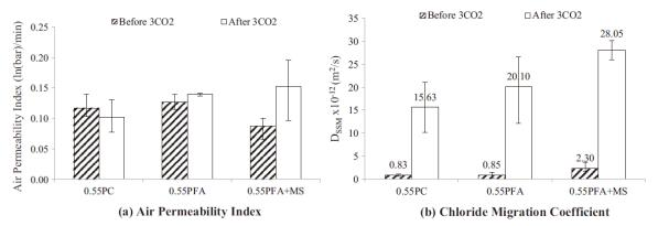
**Figure 10:** Influence of carbonation on air permeability and chloride migration coefficient of different types of concrete [41]
