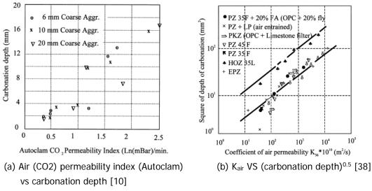
Figure 6: The relationship between carbonation and air permeability
