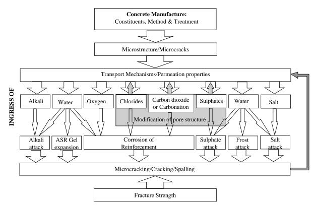
Figure 2: Dependence of durability of concrete on microstructure and transport mechanisms [7]
