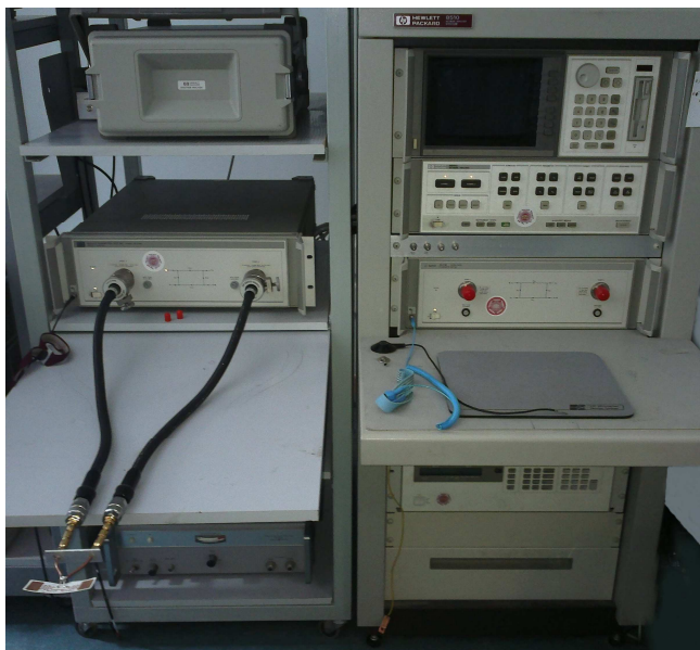
Figure 3 Measurement setup using Agilent HP8510C network analyzer.
