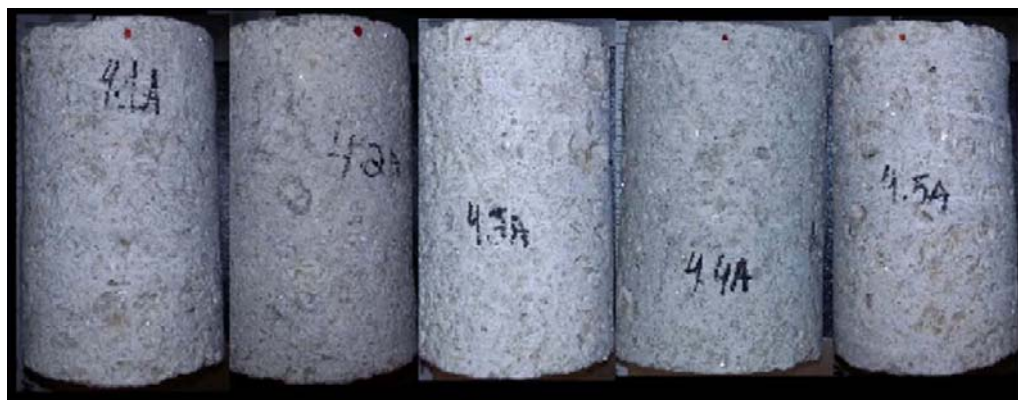
Figure 2 – 4A series studied. Naked eye analysis allows the observation of some vuggy or moldic porosity on the surface of the plugs.
