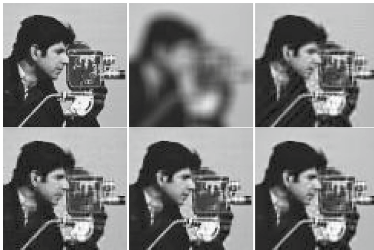
Fig. 1 Deblurring of Cameraman image, scenario 3. From left to right and from top to bottom are presented zoomed fragments of the following images: original, blurred, and noisy, reconstructed by BM3DDEB, L0-Abs, IDD-BM3D, and our method. In our method, the two input parameters (\sigma, s) , are (7.5, 550) for this scenario, (7.5, 85) for scenario 1, (7.5, 25) for scenario 2, (7.5, 10) for scenario 4, (7.5, 50) for scenario 5, and (7.5, 5) for scenario 6
