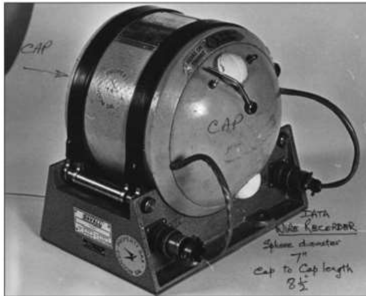
Figure 1 – The Davell Type 1050 Flight Data Recorder, or ‘Davell Red Egg’, so called because the London clock making firm of S. Davall & Sons Ltd manufactured it and its (red coloured) spheroid shape contained an improved magnetic wire recorder. The shape was adopted due to its location in the unpressurised tail sections of early jet airliners, and to give it sufficient strength to be crash survivable. This was the first commercial Flight Data Recorder (Source: Campbell, 2007).
