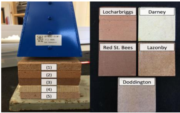
Fig. 3. Stacked sandstone arrangement for saturated layer proximity test (numbered positions shown)
