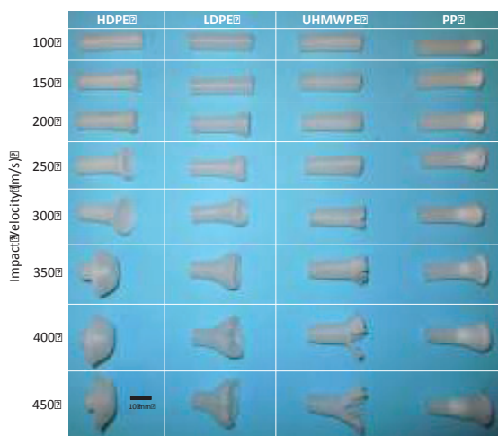
FIGURE 3. Composite of images from HDPE, LDPE, UHMWPE and PP following impact experiments at velocities between 100 and 450 m/s. The black scale bar (lower left) is 10 mm.
