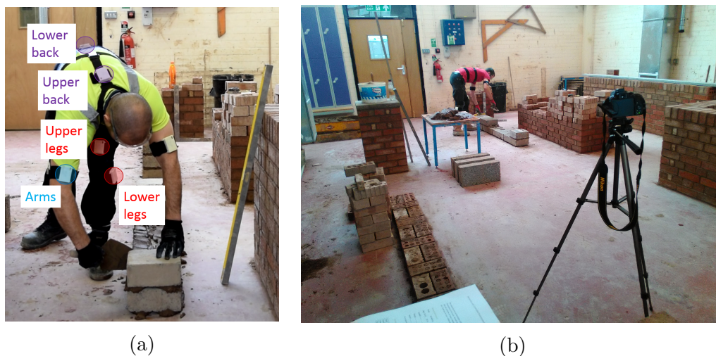
Figure 1: (a) Location of AT-BAN sensors on the body. (b) Set up of the system.
