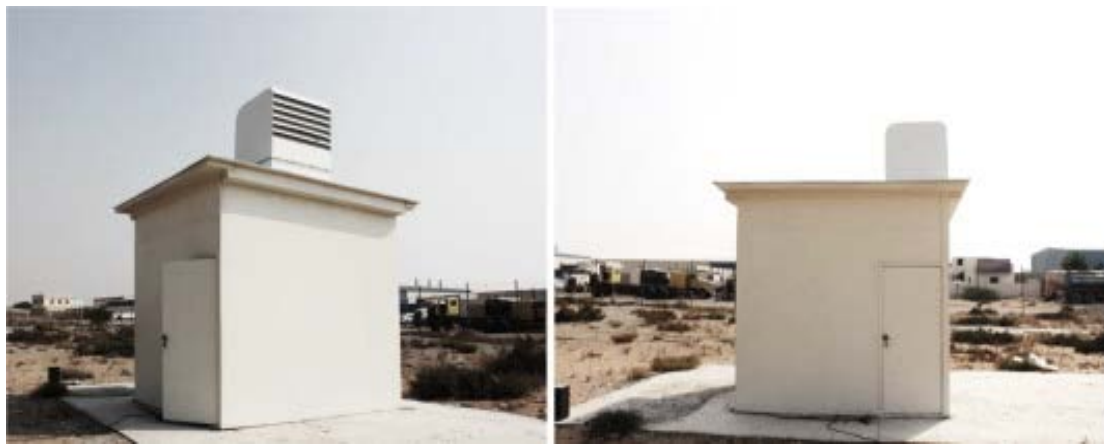
157 Figure 2 Field testing of passive cooling windcatcher with heat pipe arrangements [23]
