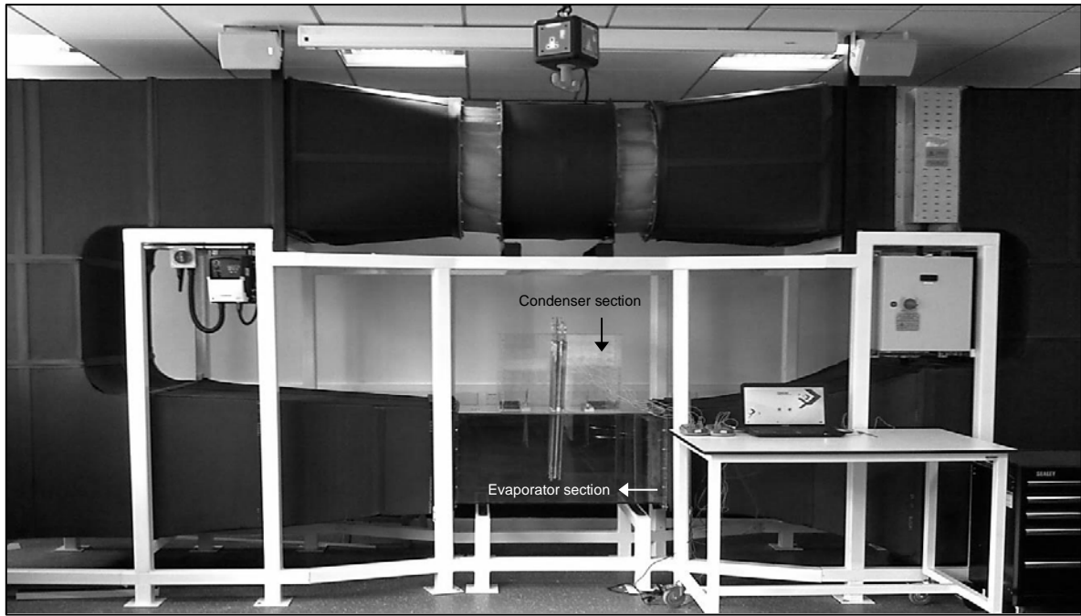
Figure 6 Closed-loop wind tunnel showing the experimental set-up for heat pipe testing
