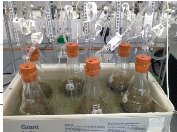
Figure 2: Semi-batch anaerobic digester set up
