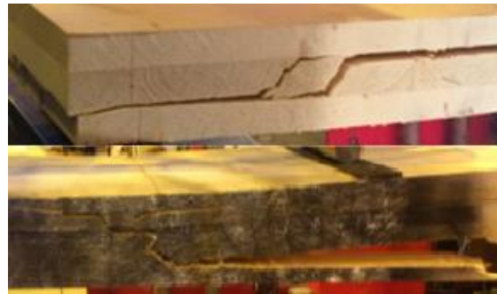
Figure 3. Rolling shear failure of 3-layer (top) and flexural failure of 5-layer samples (bottom).
