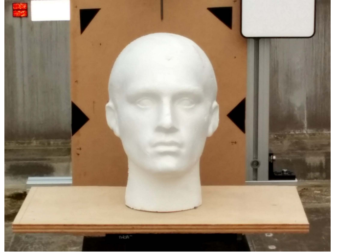
Fig. 4. Photograph showing the polystyrene head used for the experiments described here and calibration targets, including the Spectralon panel (top right corner).
