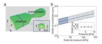
Fig. S1 Stability of microconstriction dimensions during pressure application:
