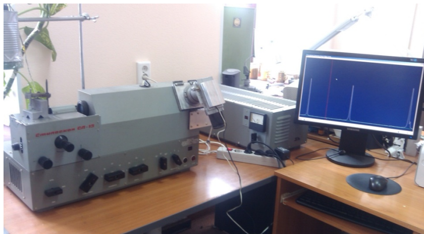
Figure 1. Exterior view of a steeloscope with photoelectric registration
